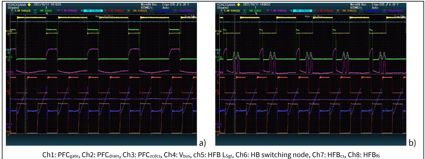
Figure 14 Continuous operation mode with HFB in CRM at 28 V, 5 A output: a) PFC switching at first valley at 90 V input, and b) PFC switching at third valley at 115 V input
