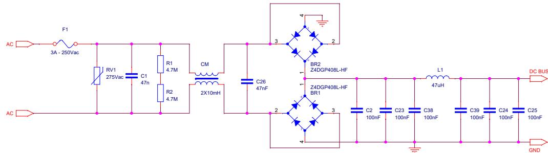
**Figure 4. Main board circuit schematic**
