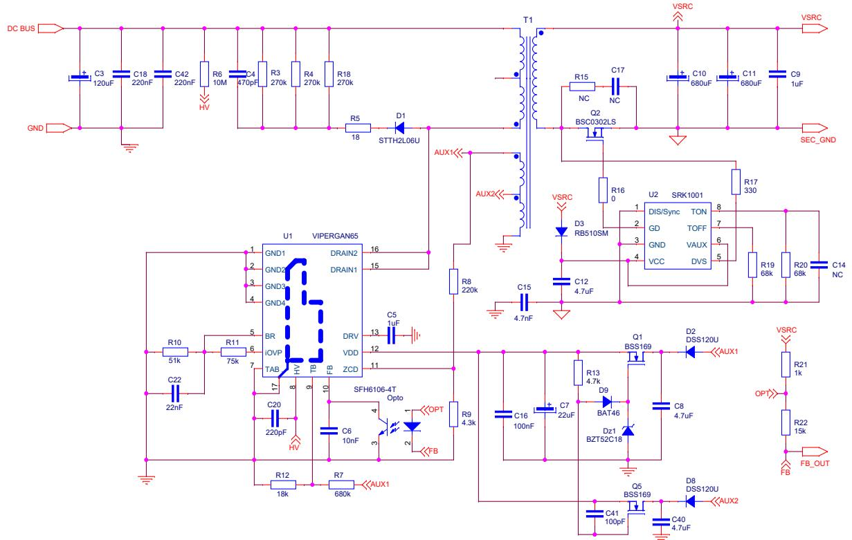
**Figure 5. Daughterboard circuit schematic**
