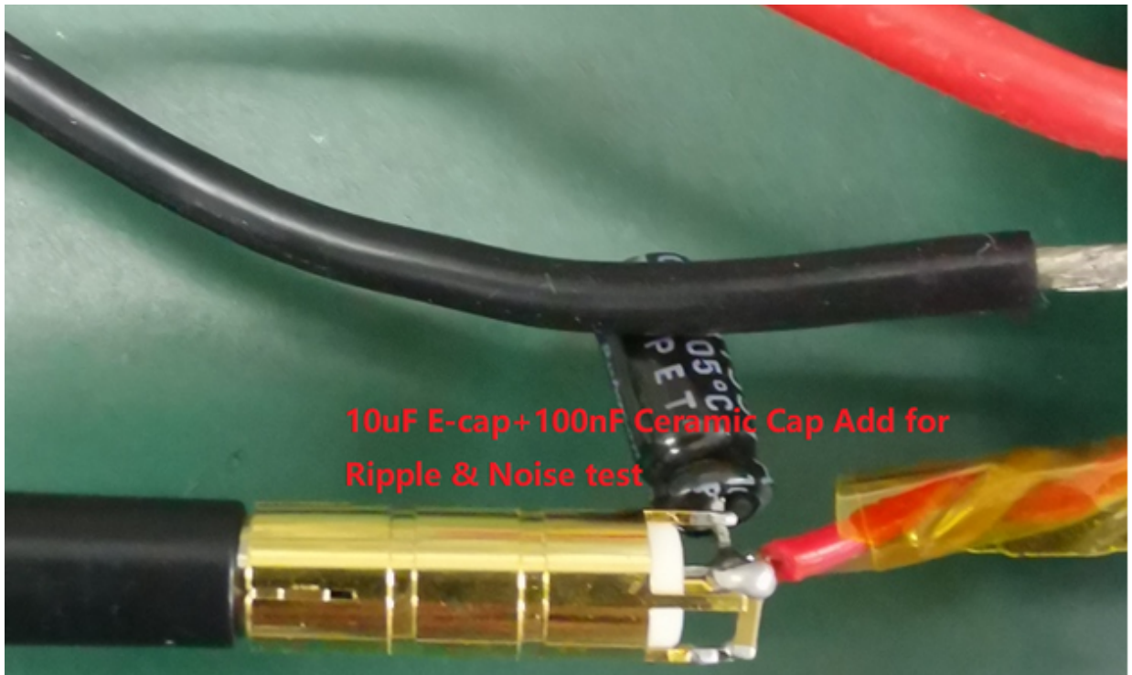
Figure 7. STDES-65ACFADP ripple and noise test setup
