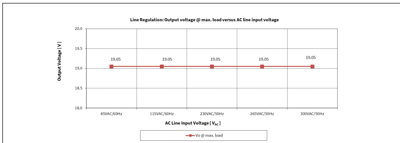
Figure 10 Line regulation V_{out} at full-load vs AC-line input voltage
