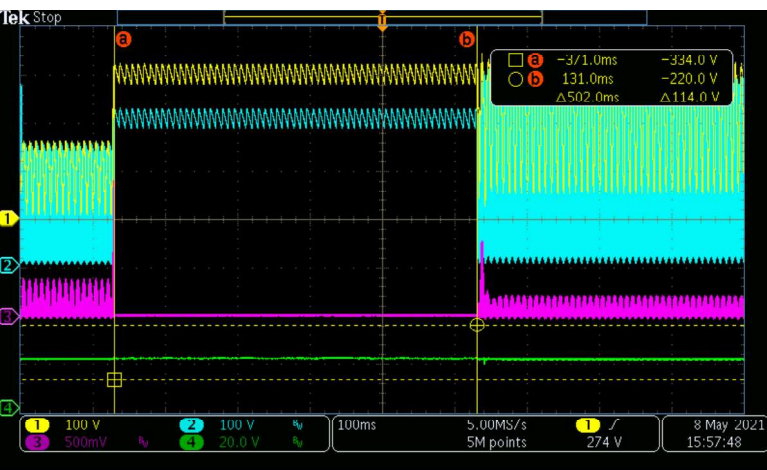
115Vac to 230Vac at 20V5A
