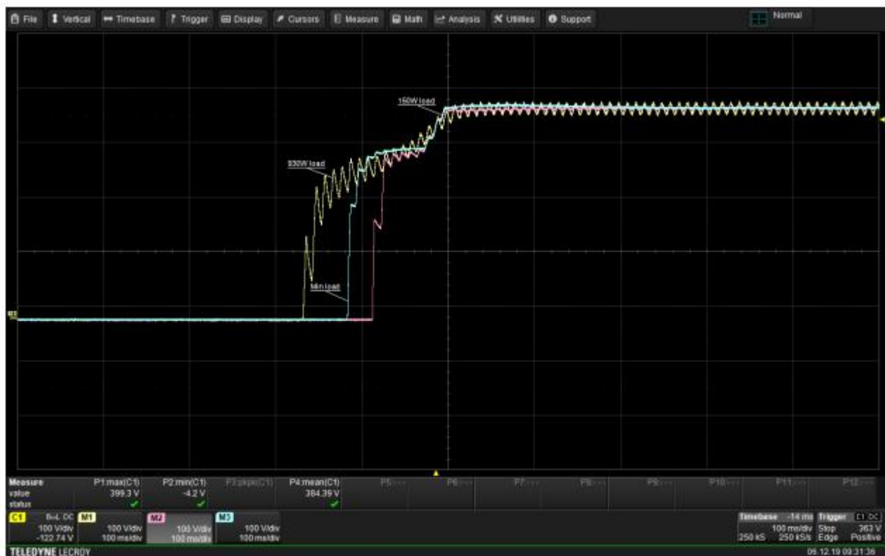
Figure 11. Start up to Open Circuit, 155 W and 930 W at 230 V AC Input
