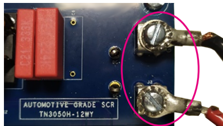
Figure 9. STEVAL-DPSTPFC1 output HVDC connection
