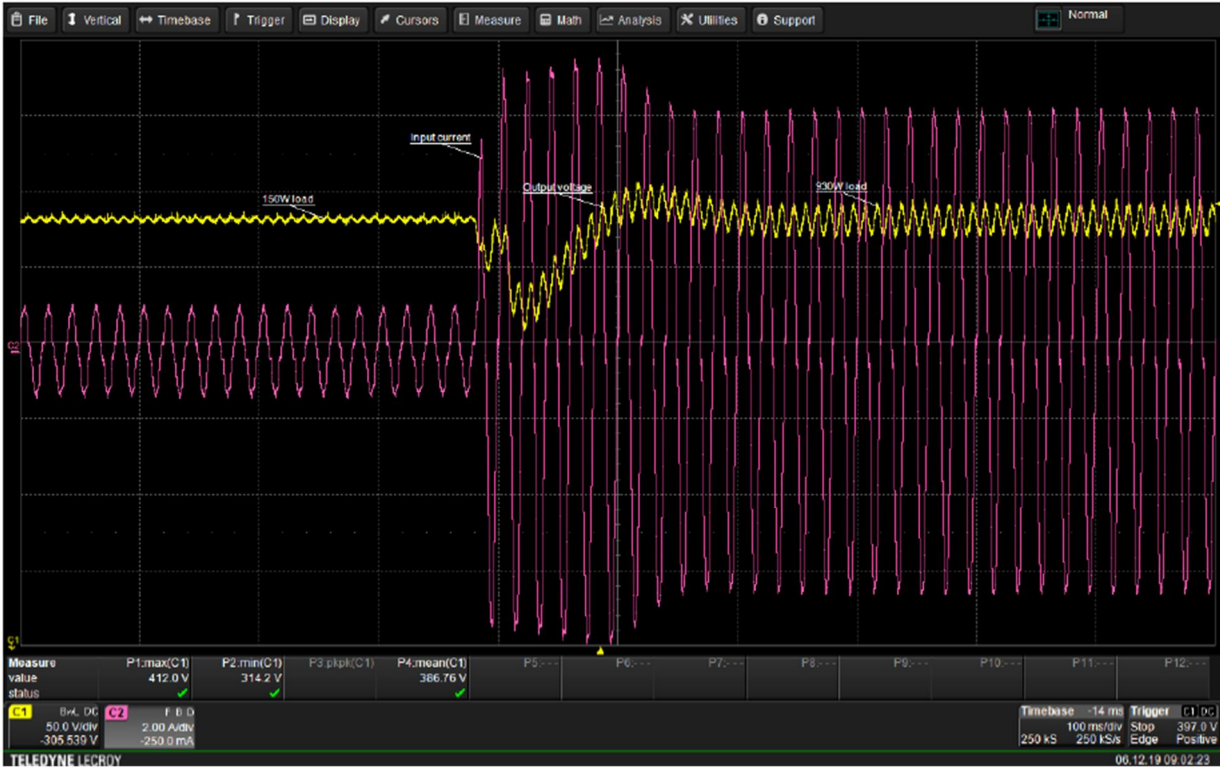
155W to 930W 之負載變動波形(C1:輸出電壓,C2:輸入電流)
