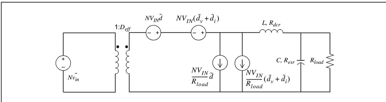
The output voltage to duty cycle transfer function,  $G_{vd}(s)$ , is given by [Equation 45](#).
