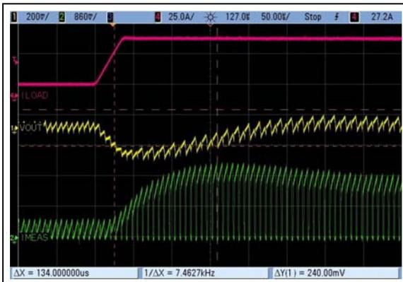
Figure B-7 shows a magnified version of the load throw-off transient of 75%-15% load. The figure also shows the settling time and the peak undershoot during the load throw-off transient.
