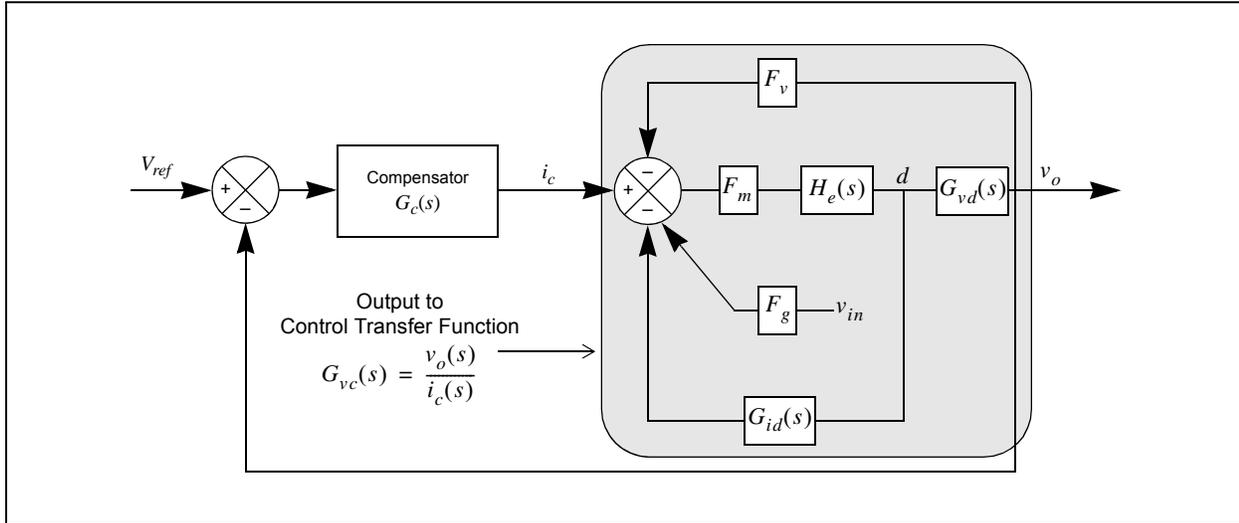
The expression for output voltage to control input,  $G_{vc}(s)$ , is obtained in Equation 59.
