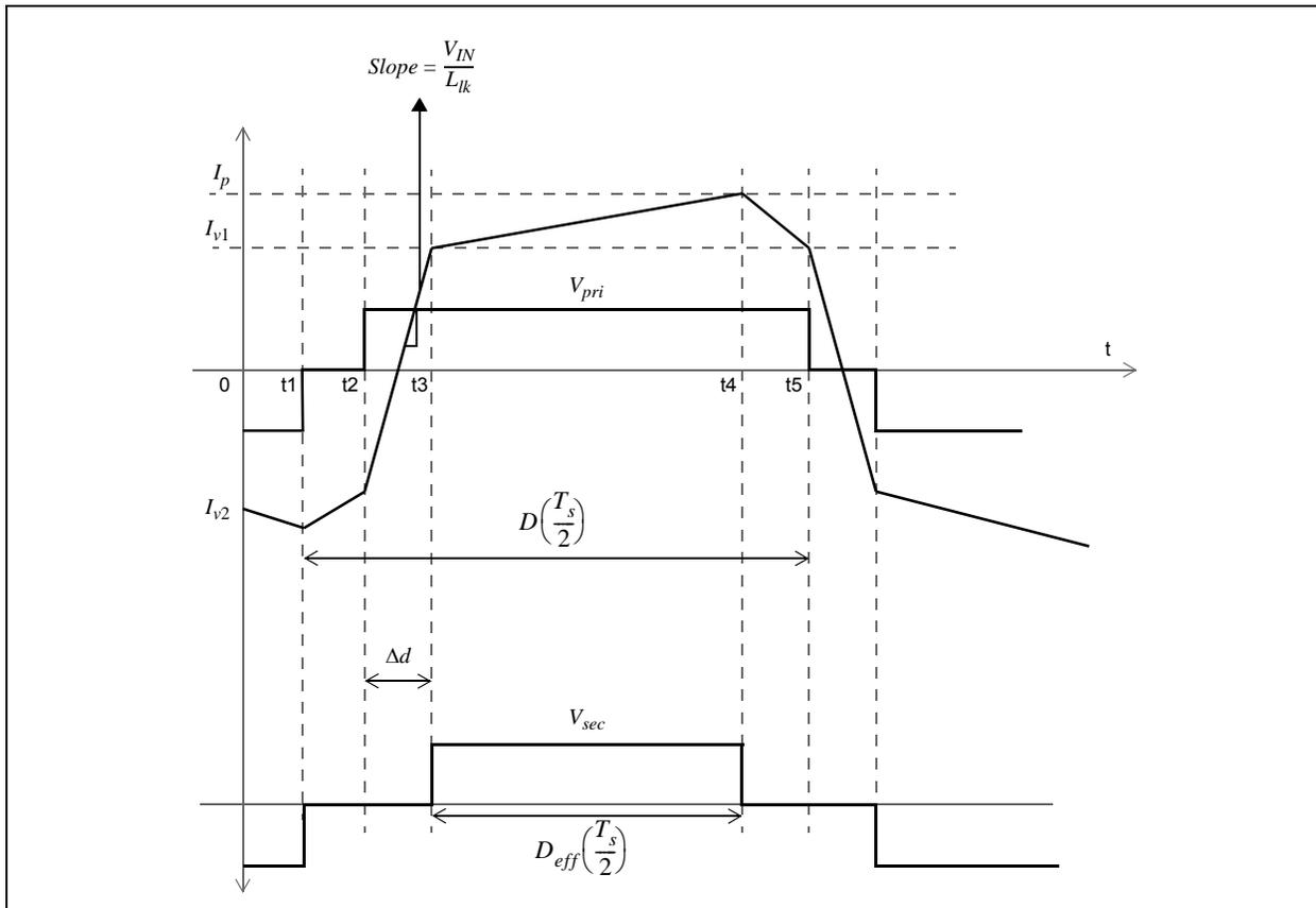
In [Figure 15](#), it is observed that the duty cycle seen in the secondary side of the transformer is lower than the duty cycle seen in the primary side. When the diagonal switches turn on, starting the power delivery cycle, the transformer current ( $i_{pri}$ ), reverses direction with a slope defined by [Equation 32](#).
