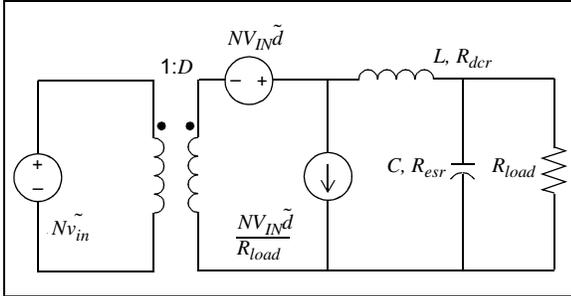
Replacing  $\tilde{d}$  with  $(\tilde{d}_{eff})$  in [Figure 16](#) results in showing the small signal model of the ZVS FB Converter and the dynamics consideration due to the resonant inductor, as shown in [Figure 17](#). The small signal model for the ZVS FB Converter is shown in [Equation 44](#).
