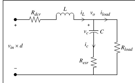
A small signal model of a buck derived converter can be represented in the state-space form and is shown in Equation 28.
