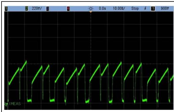
Figure B-4 shows the sensed current waveform with the application of a digital slope compensation algorithm to the voltage compensator output. From the waveform in Figure B-4, it should be noted that the effective duty cycle is ~80%. It can be concluded that the digital slope compensation algorithm is effective in eliminating the subharmonic oscillations due to duty cycles > 50%, resulting in a smooth steady-state current.
