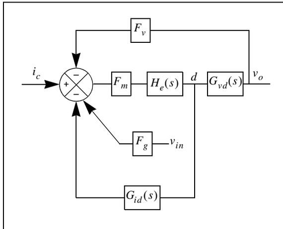
In Figure 20, the high-frequency model term,  $H_e(s)$ , is given by Equation 58.
