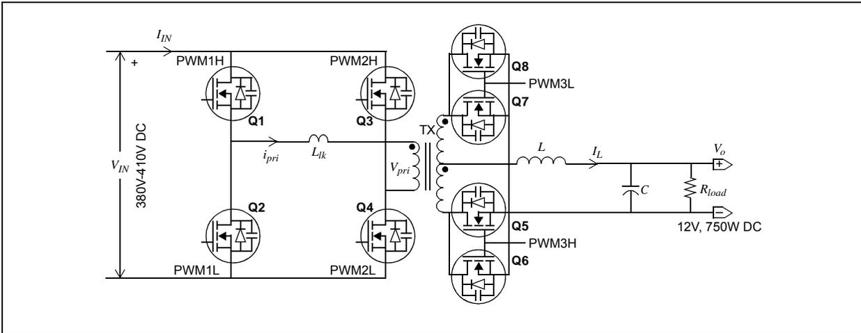
**FIGURE 2: PEAK CURRENT CONTROL – ANALOG**
