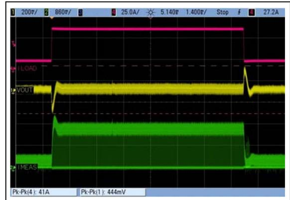
Figure B-6 shows a magnified version of the loading transient of 15%-75% load. The figure also shows the settling time and the peak undershoot during the loading transient.
