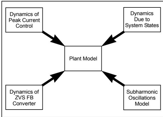
In the following sections, each component is separately derived and then integrated to obtain the overall plant model that can be used to design a suitable compensator. In a peak current controlled system, the output variable to be controlled is the output voltage,  $v_o$ , and the control variable is the peak current reference,  $i_c$ . Therefore, the target plant model is to obtain the s-domain transfer function relating to the output voltage and the peak current reference.
