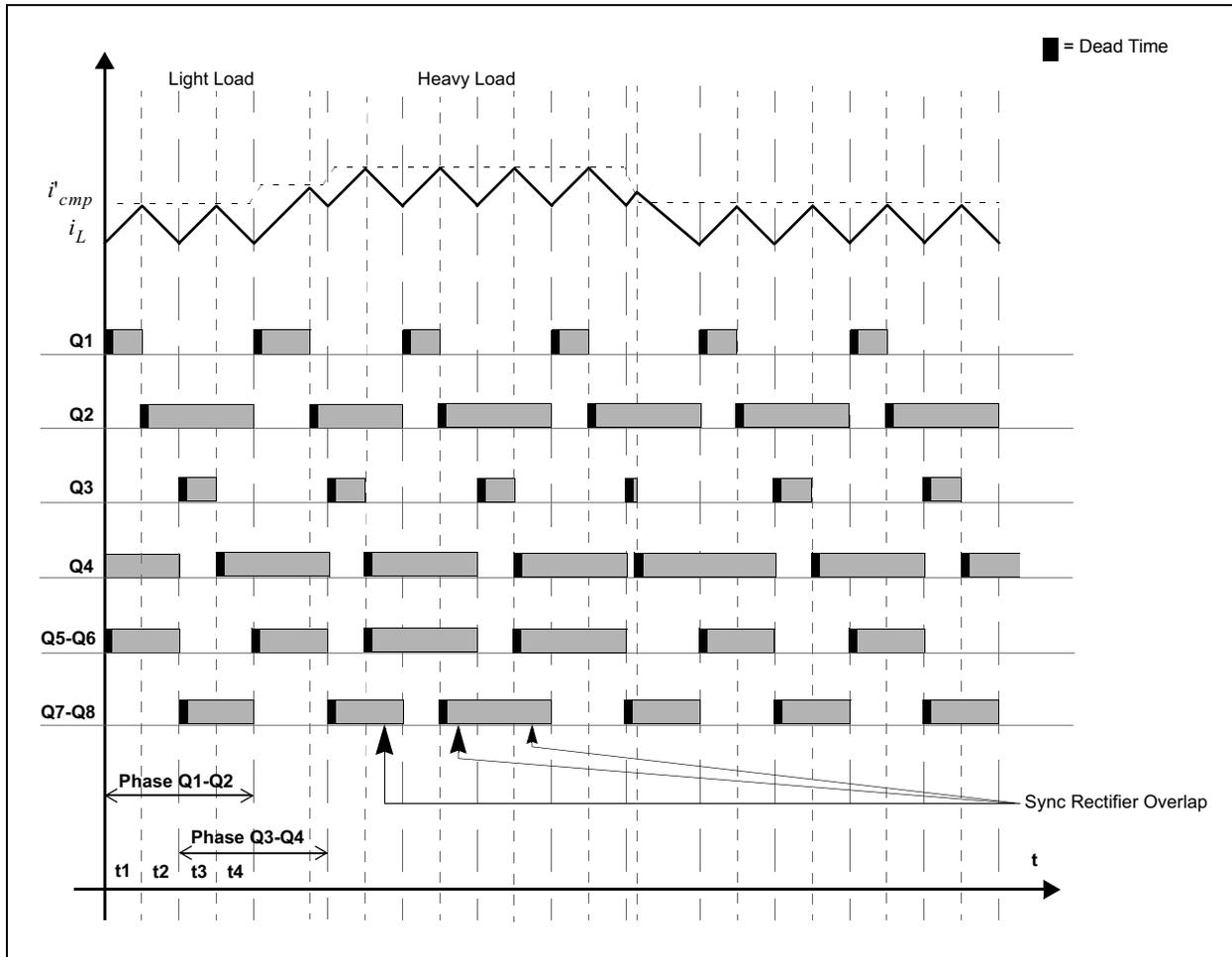
For achieving synchronous overlap, the following settings are needed for configuring the PWM Generator, which provides the drive signals for the synchronous MOSFETs:
