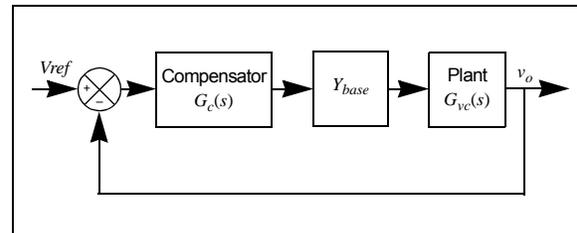
The nominal values of the components of the plant are given in Table 2. By substituting these component values in Equation 45 and Equation 46, the plant transfer function with  $Y_{base}$  (Equation 60) is obtained.
