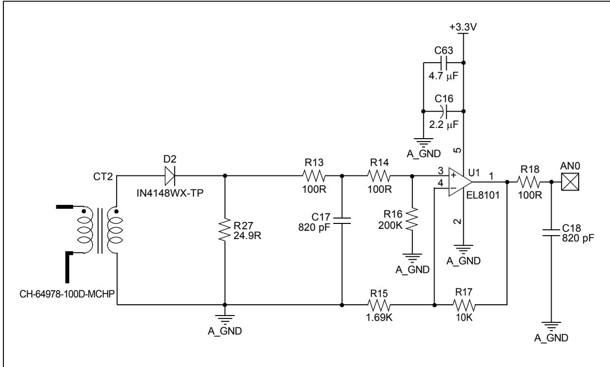
Figure 7 shows two low-pass filters: one at the input of the amplifier and another at the output of the amplifier. The corner frequency of the resulting second order filter has been chosen, such that it eliminates the high-frequency switching noise present in the current waveform. The filter stage transfer function is given by Equation 2.
