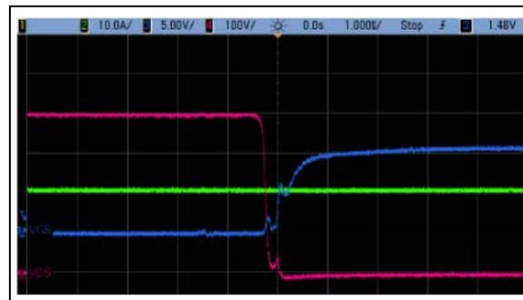
Figure B-10 shows the drain to source voltage (VDS) and the gate to source (VGS) voltage of a Q2 MOSFET at a 50% load. This figure also depicts the ZVS turn-on at the beginning of the t2 interval, as shown in Figure 4.
