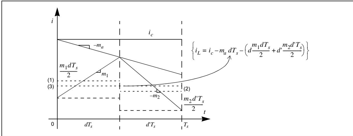
From [Figure 12](#), the average of the first triangular portion of the inductor current (corresponding to the slope,  $m_1$ , and the interval  $dT_s$ ) is given by:  $\frac{m_1 d T_s}{2}$
