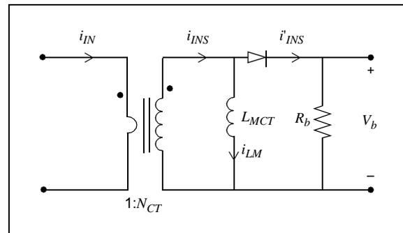
The aim is to minimize the magnetizing current,  $i_{LM}$ , to obtain a true reflection of the primary current ( $i'_{INS} \approx i_{INS}$ ). The magnetizing current is directly proportional to the voltage across the secondary terminals and inversely proportional to the square of the secondary side turns of the CT ( $i_{LM} \propto \frac{V_b}{N_{CT}^2}$ ).
