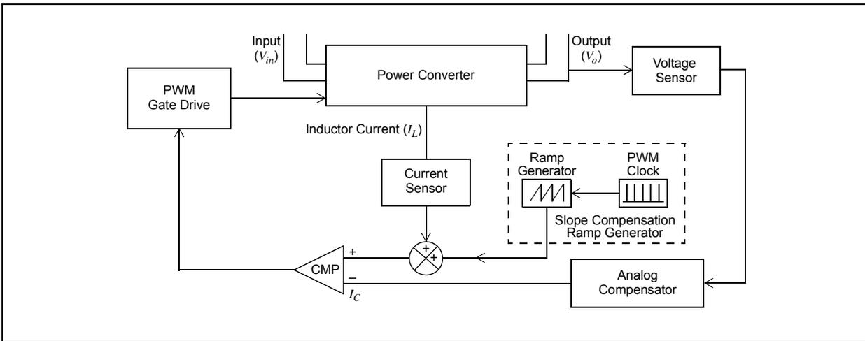
**FIGURE 3: PEAK CURRENT CONTROL – DIGITAL**
