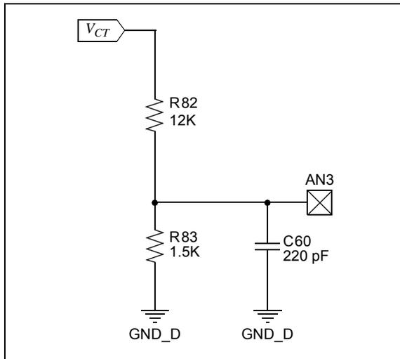
The gain of the input voltage sensor has to be chosen to cover input voltages up to 450V for a greater dynamic range. For a transformer (TX) turns ratio of 25:1:1 ( $K_{VIN}$ ), the gain for a full-scale voltage of the ADC pin is given by the expression,  $ADC\_REF/VIN\_MAX/N$ , which translates to a value of 0.1833.
