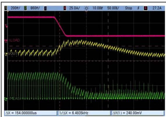
From Figure B-6 and Figure B-7, it can be observed that the subharmonic oscillations are eliminated from the current waveform, even during load transients.
