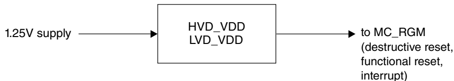
Figure 5-1. Logic scheme of the core voltage detectors
